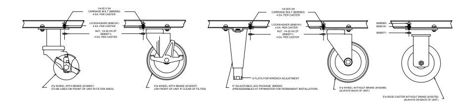
WHETHER INSTALLING CASTERS OR LEGS ALWAYS USE 4 EA. 1/4-20 X 3/4 CARRIAGE BOLTS (8090563) WITH 4 EA. LOCKWASHERS (8090191) FOR EACH CASTER OR LEG ASSEMBLY AND TORQUE EACH NUT TO 50 INCH LBS. MINIMUM. SEE ABOVE DIAGRAMS FOR PROPER LOCATION OF LOCKWASHWER.
